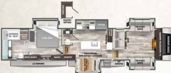
371FL HITCH WEIGHT-2,615 lb. / GVWR-16,615 lb. / UVW-13,564 lb. CCC-3,051 lb. / LENGTH-41' 11" / HEIGHT-13' 6" / WIDTH-96"
