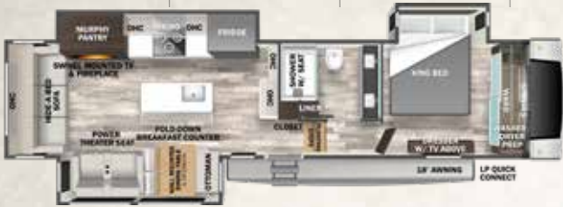
360RL HITCH WEIGHT-2,525 lb. / GVWR-16,525 lb. / UVW-13,134 lb. CCC-3,391 lb. / LENGTH-40' 7" / HEIGHT-13' 6" / WIDTH-96"
