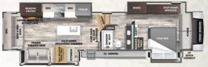
380RL HITCH WEIGHT-2,790 lb. / GVWR-18,000 lb. / UVW-14,389 lb. CCC-3,611 lb. / LENGTH-42' 10" / HEIGHT-13' 6" / WIDTH-96"
