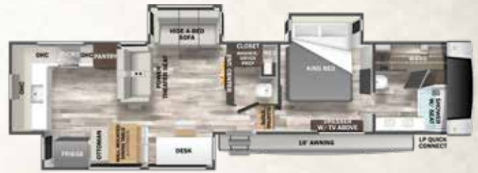
388RK2 HITCH WEIGHT-2,205 lb. / GVWR-18,000 lb. UVW-14,209 lb. / CCC-5,561 lb. / LENGTH-42' HEIGHT-13' 6" / WIDTH-96"
