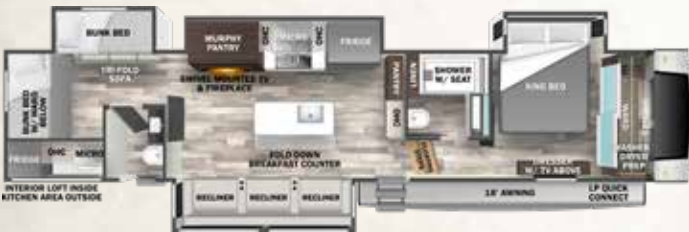
375BHO HITCH WEIGHT-2,430 lb. / GVWR-18,000 lb. / UVW-14,209 lb. CCC-3,791 lb. / LENGTH-43' 1" / HEIGHT-13' 6" / WIDTH-96"
