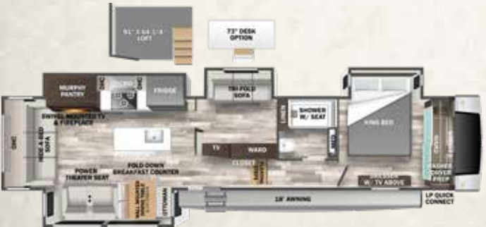
377BH HITCH WEIGHT-2,135 lb. / GVWR-16,135 lb. / UVW-12,679 lb. CCC-3,456 lb. / LENGTH-42' 5" / HEIGHT-13' 6" / WIDTH-96"
