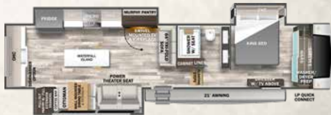
391WOW HITCH WEIGHT-TBD / GVWR-18,000 lb. UVW-TBD / CCC-TBD / LENGTH-43' 2" HEIGHT-13' 6" / WIDTH-96"
