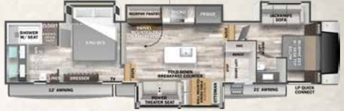
380MUD HITCH WEIGHT-2,555 lb. / GVWR-18,000 lb. / UVW-14,739 lb. CCC-3,261 lb. / LENGTH-43' 5" / HEIGHT-13' 6" / WIDTH-96"
