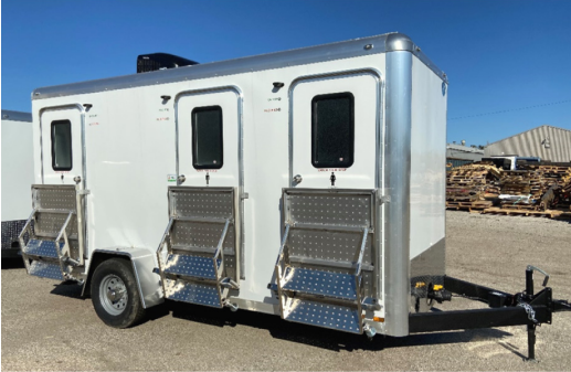
View Of The Trailer With Steps And Porches Retracted. The Railings Are Stored In The Mechanical Room
