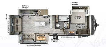
LENGTH: 36' 8" WIDTH: 8' HEIGHT: 11' 7" HITCH: 1375 AXLE: 8020 UVW: 9454 CCC: 1921 6 54 GAL 6 122 GAL B 53 GAL
